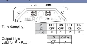
Switching level setting by way of voltage on MB:
