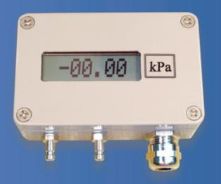
These pressure transducers are designed for low and very low pressures and pressure differences measuring. They may be used in wide application in a branch of air-conditioning, ventilation, combustion process control, clean rooms monitoring, equipment design, etc. These transmitters can measure positive and/or negative pressure differences or overpressure and/or underpressure against ambient atmosphere, eventually measuring of absolute or barometric pressure.
